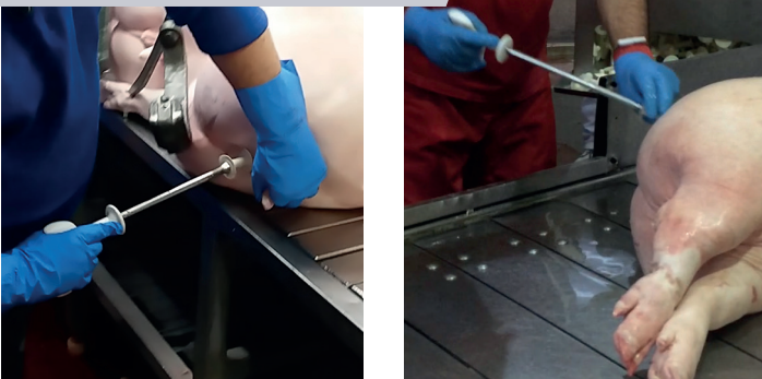
Plugs being inserted on shackle conveyer
