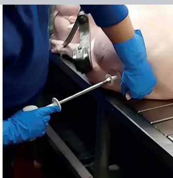
Plugs being inserted on shackle conveyer
