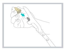
Hog Plug is loaded onto the pneumatic driven inserter tool manually by the operator or via an automated dispenser system.
